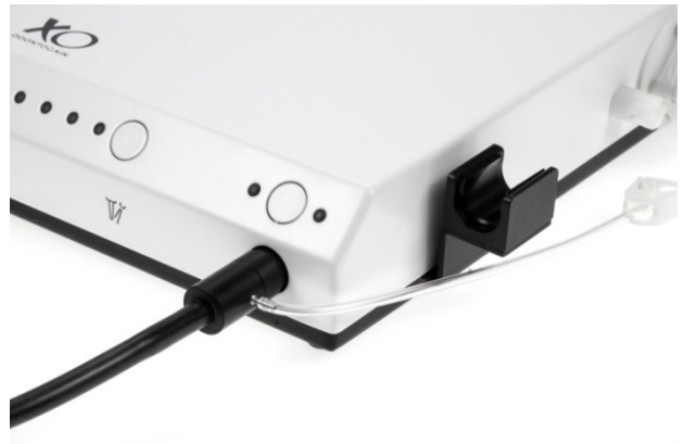
Figure 9 The other tubing from the pump wheel is connected to the irrigation inlet at the handpiece cord
