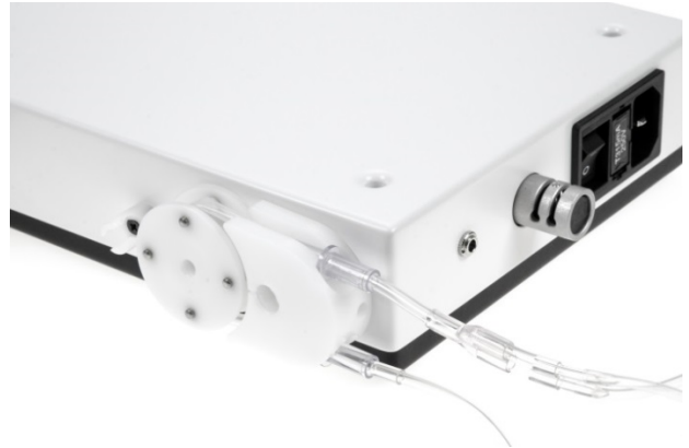
Figure 7 Tubing placed correct around the pump wheel
