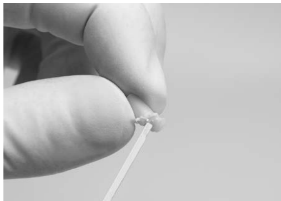
Figure 5 – Non-polymerized material is removed from composite test plug
