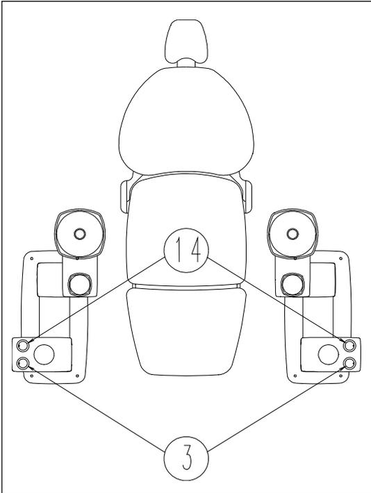
Figure 6. How to place the lamp (3) and the X-ray apparatus (14) on left and right-handed units.
