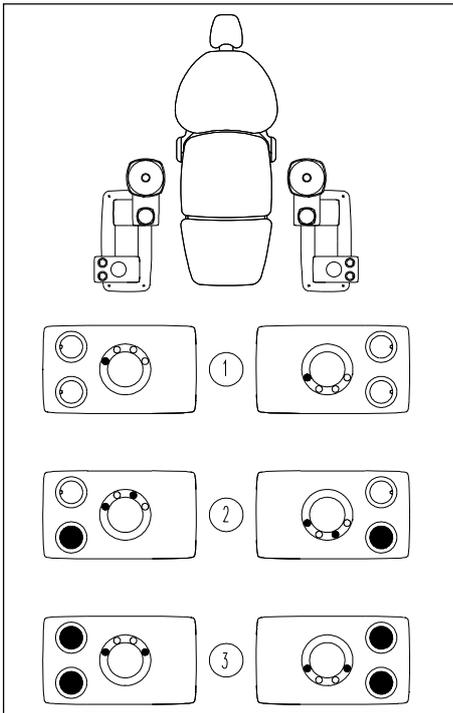
Figure 2. Stop pin positioning for left or right handed units:
